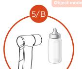
Point thermometer to object 1-5mm away and press for measurement
