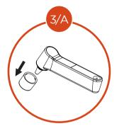
Turn on device, remove cap and thermometer will switch to ear mode automatically and **9** will be shown on screen.
