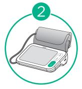
Plug the connector from cuff into the monitor on the left side
