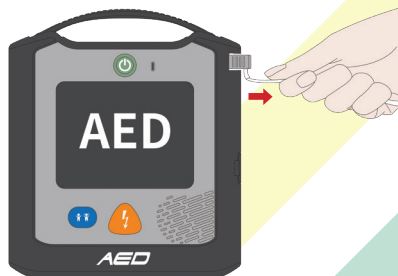
Removing the Pads connector
